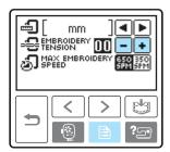
Press **–** to weaken the thread tension.
